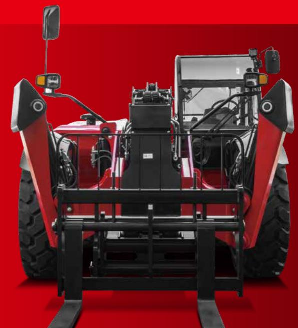
The machine is equipped with quick change device, which can realize the quick replacement of different attachments. This enables various operations including fork loading, shovel loading, clamping, aerial work, etc.
